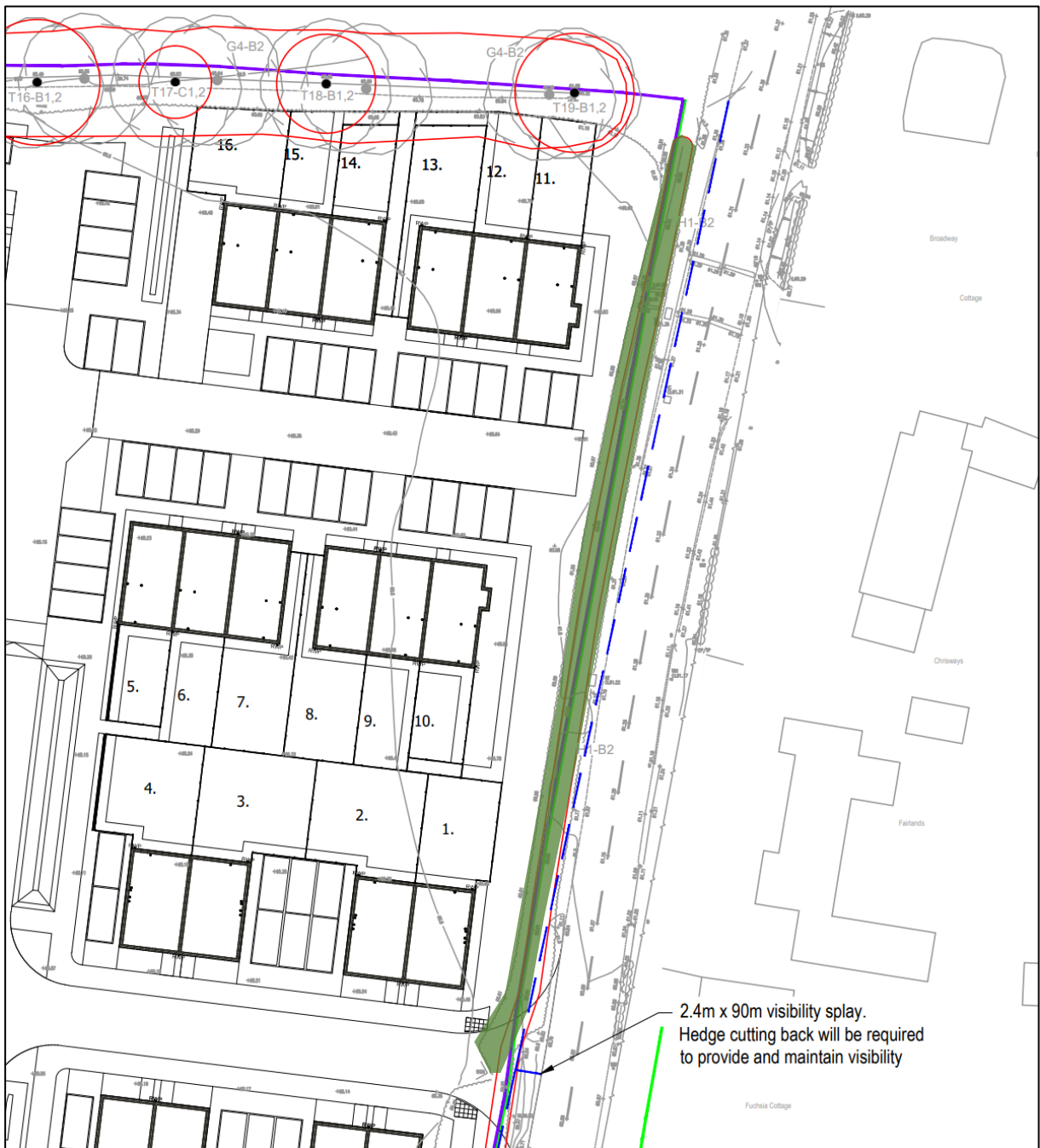
figure 12: Proposed splay [blue dashed line] north of site access and existing hedgerow [green]
